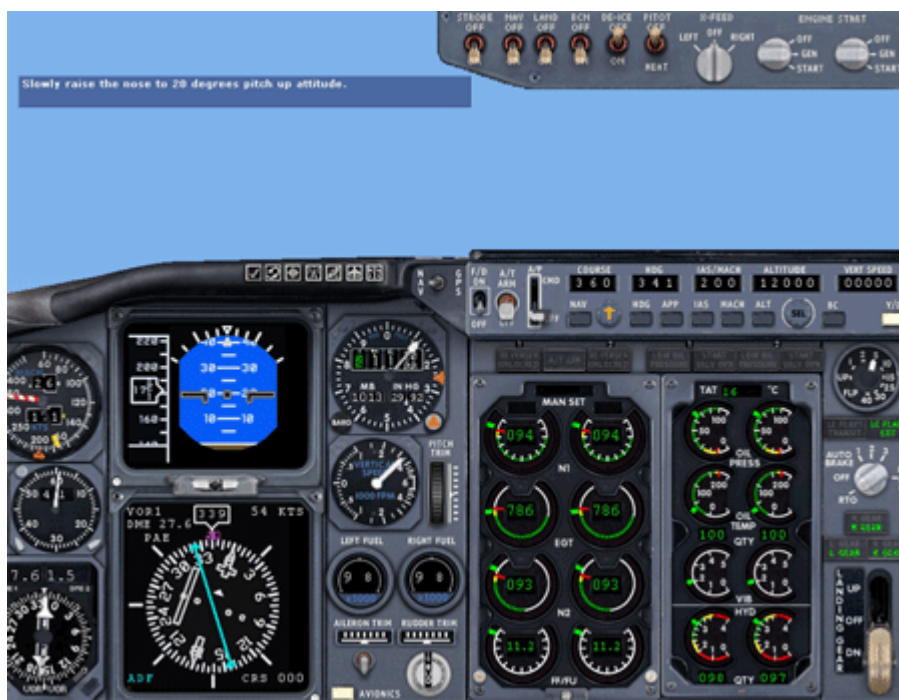
Figure 1-4: The instrument panel soon after takeoff rotation
