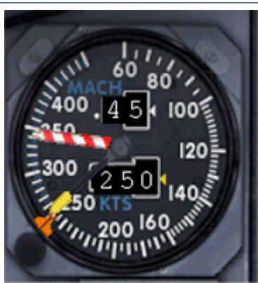
Figure 1-7: Airspeed indicator and "barber pole"
