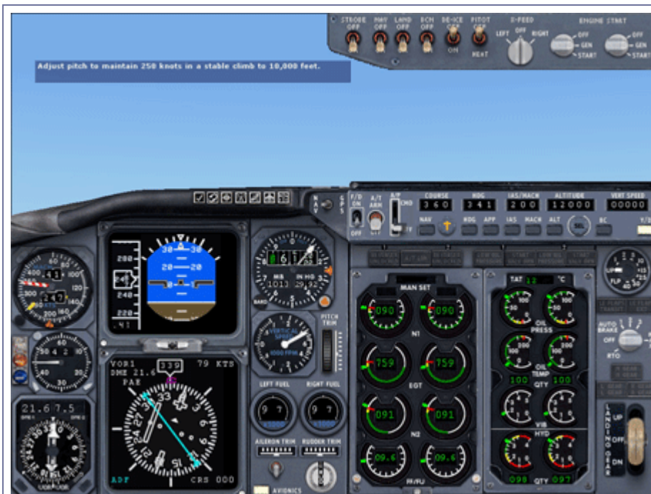
Figure 1-6: The instrument panel after retracting flaps and obtaining 12 degrees nose up pitch
