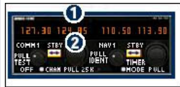
1-Standby frequency, 2-Standby flip/flop switch
